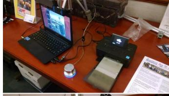
Camera plugged directly into the laptop. USB hub plugged into the other port. Printer, button, mouse (not visible) and speaker power plugged into strip in box behind the laptop.
